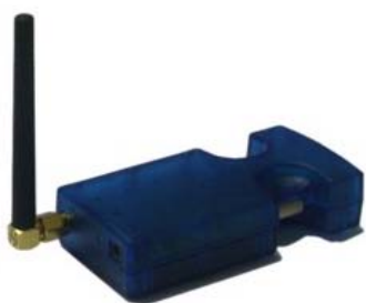
Bluetooth® device for wireless communication for the Sound Level Meter, BT001
