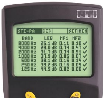
Acoustilyzer AL1 STI-PA test results of the modulation indices
